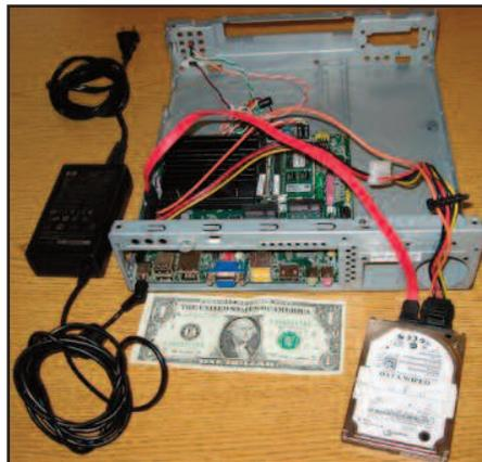
This is what we ship: DC power supply, motherboard, and hard drive with cables.
